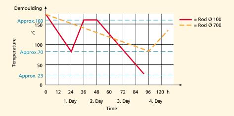
It is evident that a solid rod with Ø 100 is cooled enough to be tempered one day after demoulding. However, a solid rod with Ø 700 mm needs at least four days until it is cooled down enough for the tempering process to begin.
