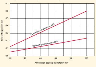
For bearing seats into which anti-friction bearings are inserted for operation at normal temperature and load conditions, we recommend the following press-fit undersizes and tolerances:
