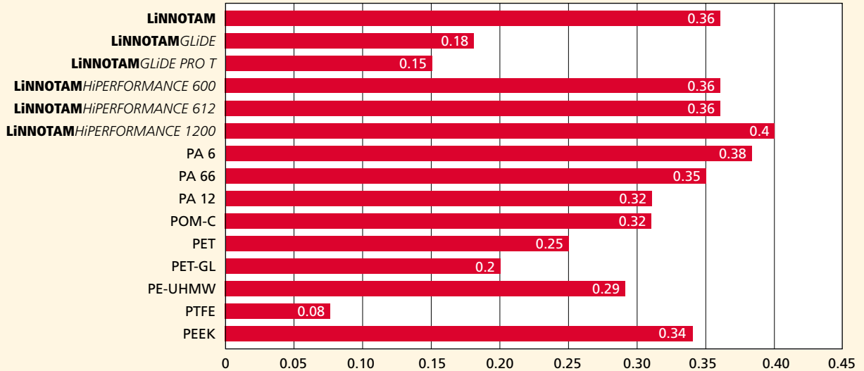
Coefficient of sliding friction against steel (hardened and ground, P = 0.05 MPa, v = 0.6 m/s, t = 60 °C in the vicinity of the running surface)
